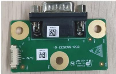
Electronic Scale Sensor Board (Top Side)
