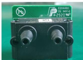
Fresh Gas Differential Pressure Sensor Board (Top Side)
