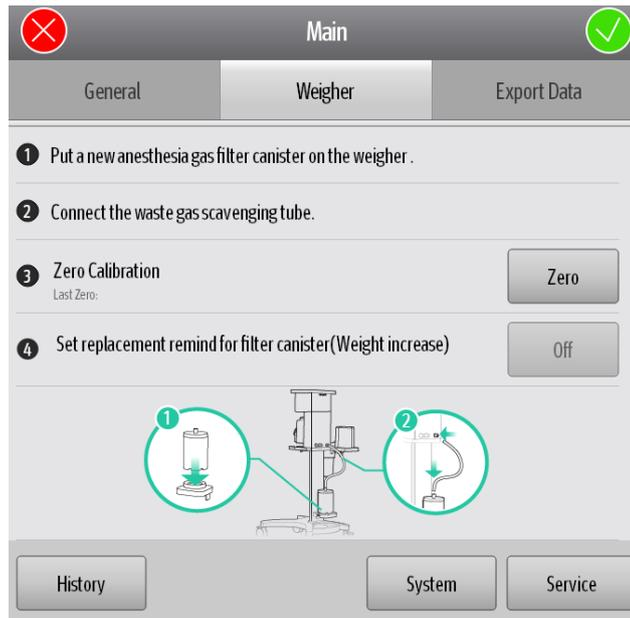
3. Place 1000 g weight on the anesthetic agent canister and confirm that the prompt "Replace Anesthesia Gas Filter Canister" appears. Remove the weight and confirm that the prompt "Replace Anesthesia Gas Filter Canister" disappears.
