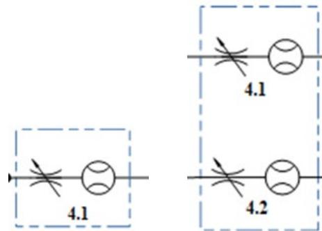
Figure 8 Principle diagram of glass tube flowmeter subsystem
