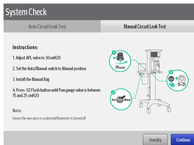
5. Ensure that the tests are passed: The system passes the automatic circuit leak test, compliance test, and manual circuit leak test.
