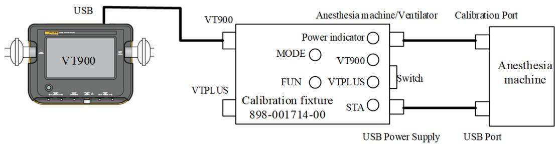
F. Select VT as the calibration device on the screen of the anesthesia machine, tap  for calibration, and wait until calibration is successful.
