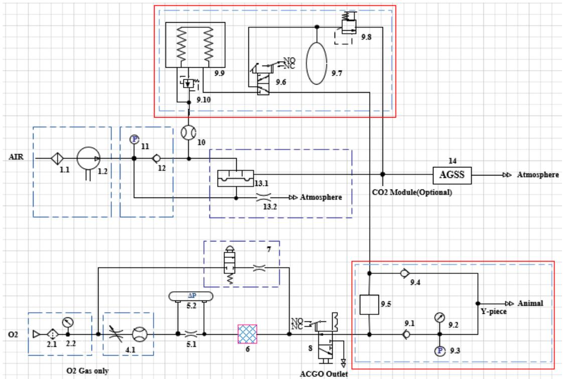
Figure 15 Principle diagram of anesthesia breathing system (Veta5)
