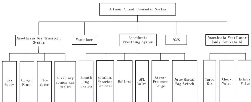
Figure 3 Structure of the Pneumatic System
