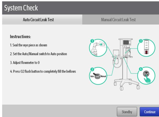
4. Follow prompts indicated on the screen to complete the manual circuit leak test.
