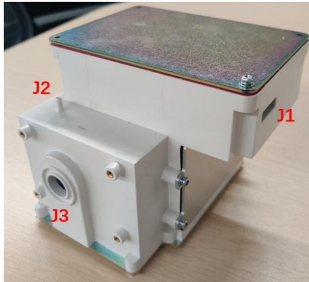
Figure 20 Structural Diagram of Blower Assembly
