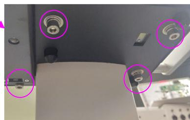
3. Use one M4×12 combination screw to fasten the snap hook to the base plate of the main unit and then insert an Allen wrench into the snap hook. The position is shown in Figure E and Figure F.
