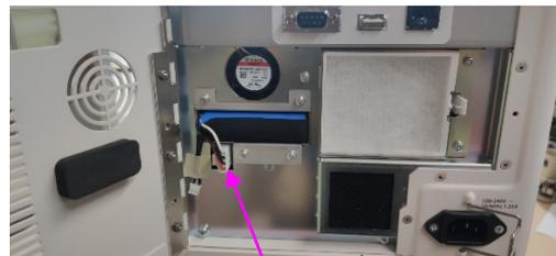
Remove the lithium battery plug.
