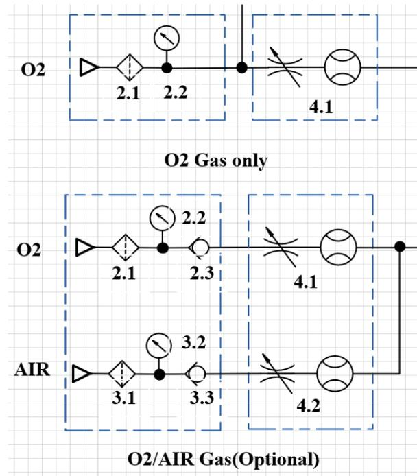
Figure 4 Pneumatic principle of the gas supply subsystem
