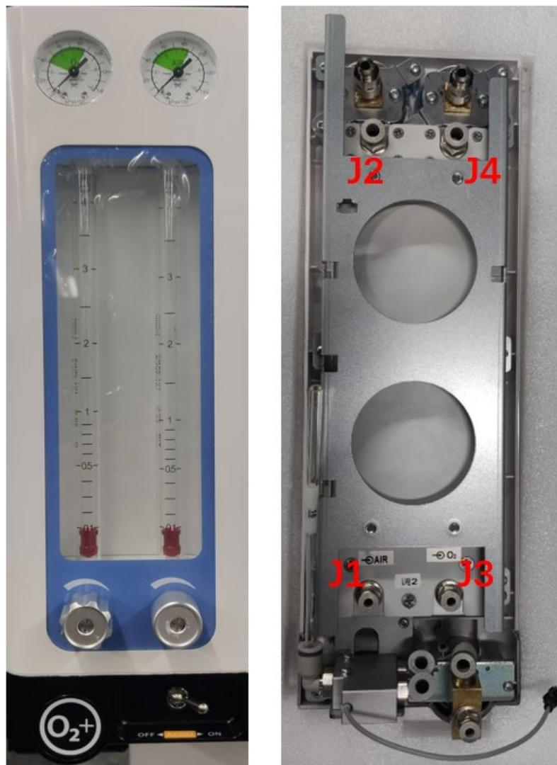
Figure 9 Structural diagram of glass tube flowmeter
