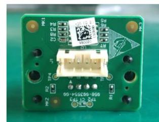
Fresh Gas Differential Pressure Sensor Board (Bottom Side)
