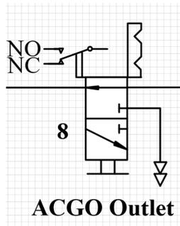
Figure 12 Principle diagram of the ACGO assembly
