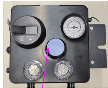
Take out the APL valve assembly upward.
