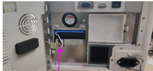
Remove the lithium battery plug.
