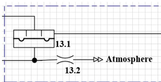
Figure 22 Principle diagram of expiratory valve assembly
