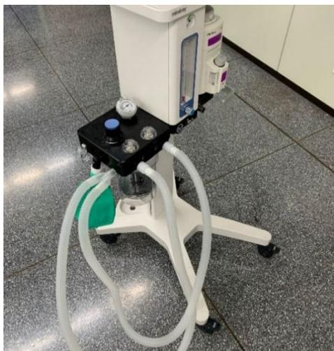
9. Adjust the APL valve to the 30 cmH<sub>2</sub>O position.
