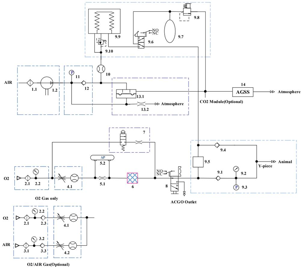
Figure 1 Pneumatic Principle Diagram (Veta 5)
