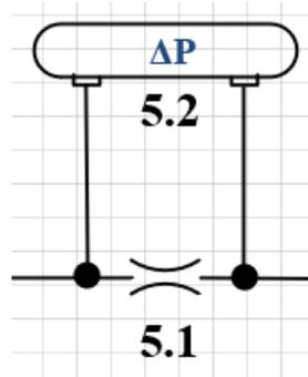
Figure 10 Principle diagram of fresh gas flowmeter
