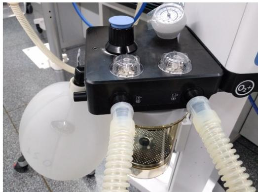
1. As shown in the figure, install the manual bag and use a corrugated hose to connect the inspiratory port to expiratory port.
