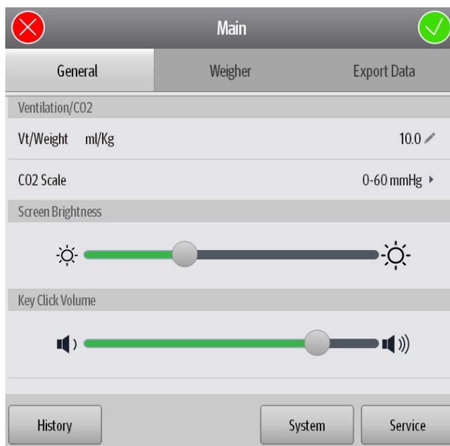
5. Close the main menu. Touch the upper left corner, lower left corner, upper right corner, lower right corner, and center of the screen separately and ensure that the keystroke sound is produced. In addition, touch the upper left corner to display the timer, touch the lower left corner to activate the weight change option, and touch the center of the screen to trigger the ventilation mode.
