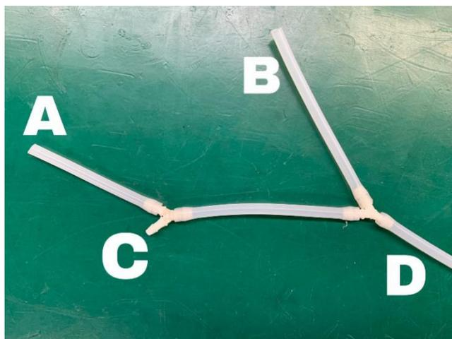
3. Connect end A to the Turbine\_P sampling port, end B to the PAW\_P sampling port, end C to the sampling tube that is originally used to connect to the Turbine\_P sampling port of the machine, and end D to VT900 (low-pressure+ end).
