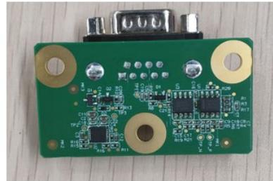
Electronic Scale Sensor Board (Bottom Side)
