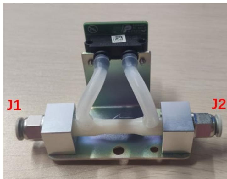
Figure 11 Structural diagram of fresh gas flowmeter
