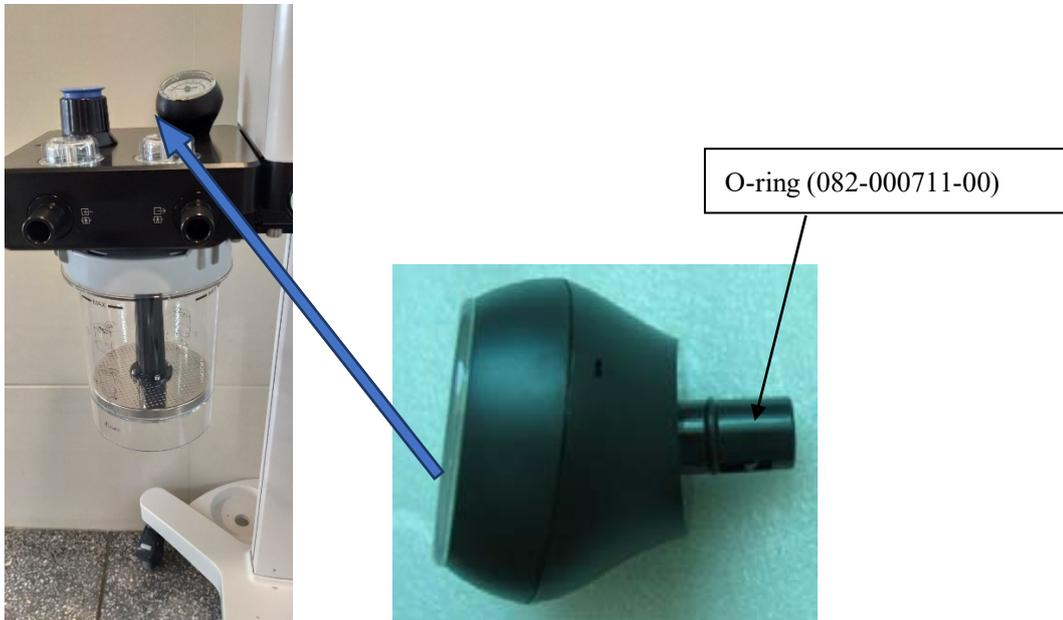
2. Replace the O-ring (M6M-010051---) of the support bracket of the CO2 absorber canister.
