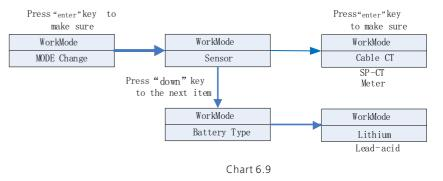
The MODE change has two options what are sensor and battery type, sensor is cable CT (default), meter and SP-CT(wireless RF transfer). In the battery type, you can choose lithium battery or lead-acid battery.
