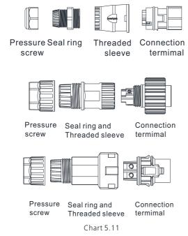
Step 2: Insert the stripped and bared cable through pressure screw, seal ring, threaded sleeve in sequence, insert cables into connection terminal according to polarities indicates on it and tighten the screws firmly. Please try to pull out the wire to make sure the it's well connected.
