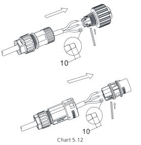
Step 3: Push the threaded sleeve into the socket, Tighten up the cap on the terminal.
