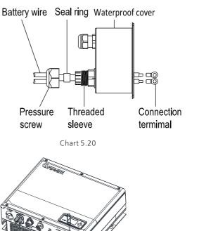
**Note:**We suggest the distance between battery and SPH no longer than 1.5m, and the power line area must be larger than 5 AWG.
