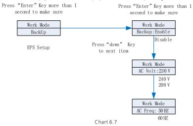
In the back up you can set EPS, including enable or disable (default is enable), AC voltage(default is 230V) and frequency (default site 50HZ).
