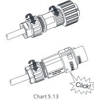
Step 4: Finally, Push or screw the threaded sleeve to connection terminal until both are locked tightly on the inverter.
