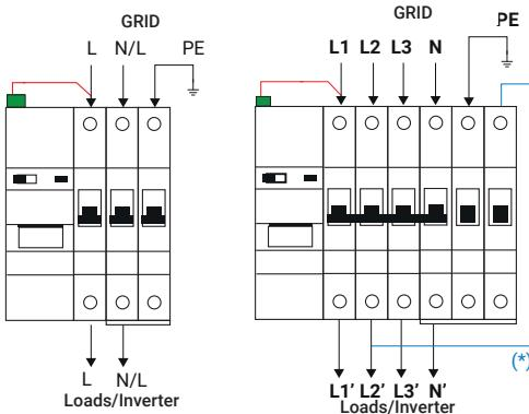
(\* ) IMPORTANT! This cable jumper must only be made on Huawei "M1" & "MB0" models.
